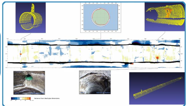
Take guesswork out of wastewater pipe inspection. In a single run, the SewerVUE MPIS Float can collect enough data to tell you the precise size and shape of the pipe, with detailed geometric information about **cracks, features, ovality**, and more.
