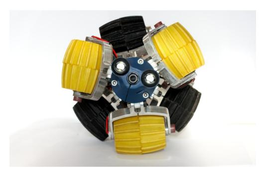
Figure 2 – The Asbestos Cement Pipe Scanner.
