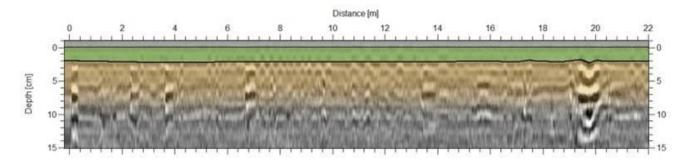
Figure 4 – PPR data from the Harbourgreene Line. Wall thickness is represented by the green-shaded area.
