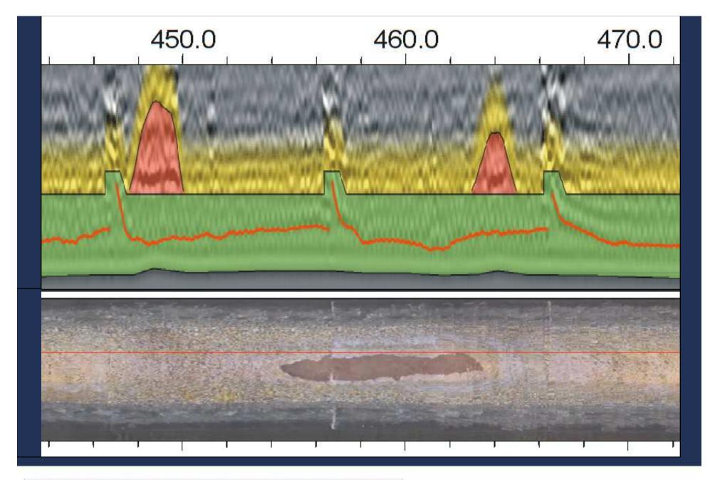
Harvard Gulch Interceptor multisensory robotic pipe condition survey including Pipe Penetrating Radar laser and CCTV Denver, CO
