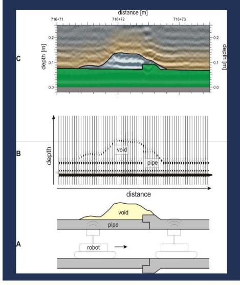
A high frequency EM wave (25 MHz to 2.5 GHz), is emitted via an antenna into the ground or structure under evaluation.
